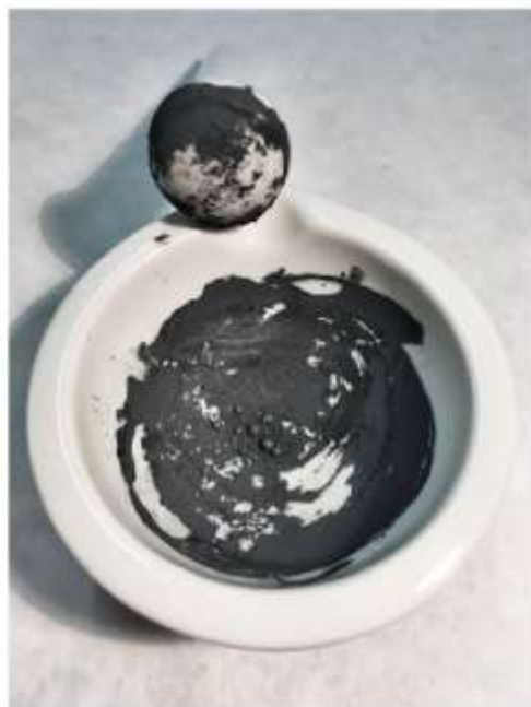
Fig. 1. Left , ceramic mortar in which HgS and copper powder were ground—droplets of mercury are visible at the bottom. Right , comparison between the XRPD pattern (blue solid line) of the residual powder obtained from the reaction of synthetic mercury sulfide and copper powder in the presence of acetic acid (reaction mixture ground with a ball mill for 4 h at 25 Hz; the high background in the pattern is due to the presence of the amorphous phase of metallic mercury in the final powder) and the XRPD pattern of synthetic mercury sulfide (red solid line). The asterisks in the red XRPD diffractogram indicate the peaks assigned to cinnabar. Phase identification was performed using the PDF 2 Release 2004 database.
